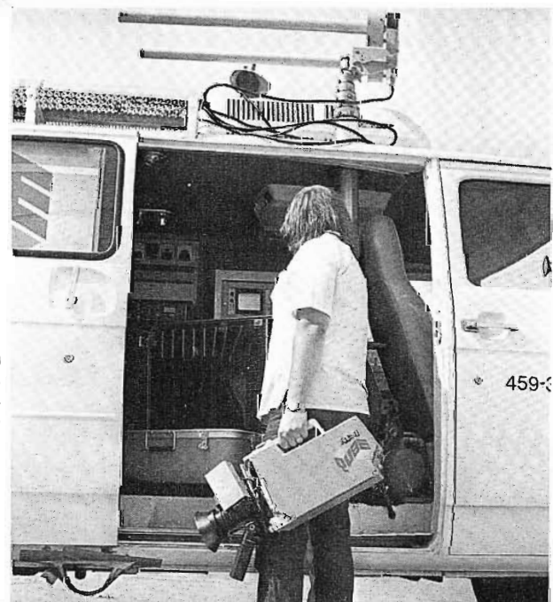
ENG unit, TK-76, and cameraman unload for a local, live pick-up. The telescoping Nurad antenna allows quick signal alignment.
